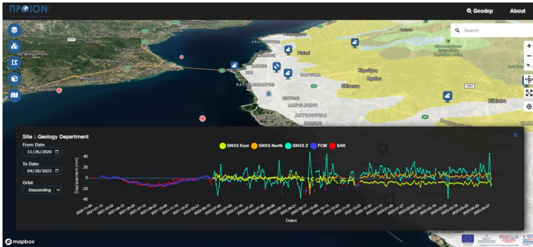
Figure 7. Time series of the GNSS, SAR observations and FCM vertical predictions of the monitoring site of Patra’s University Geology Department, visualized as a multiline-dataset line chart.
