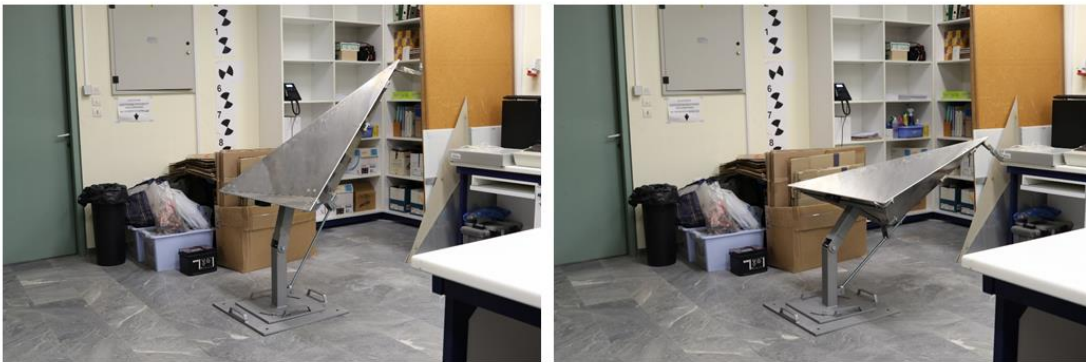
Figure 2. a) Initial position of the baseplate (5 degrees angle opening), b) Position of the baseplate (angle opening at 80 degrees).
