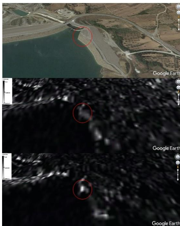
Figure 6. Identification of the corner reflector installed on Asteri dam in Sentinel-1 imagery.
