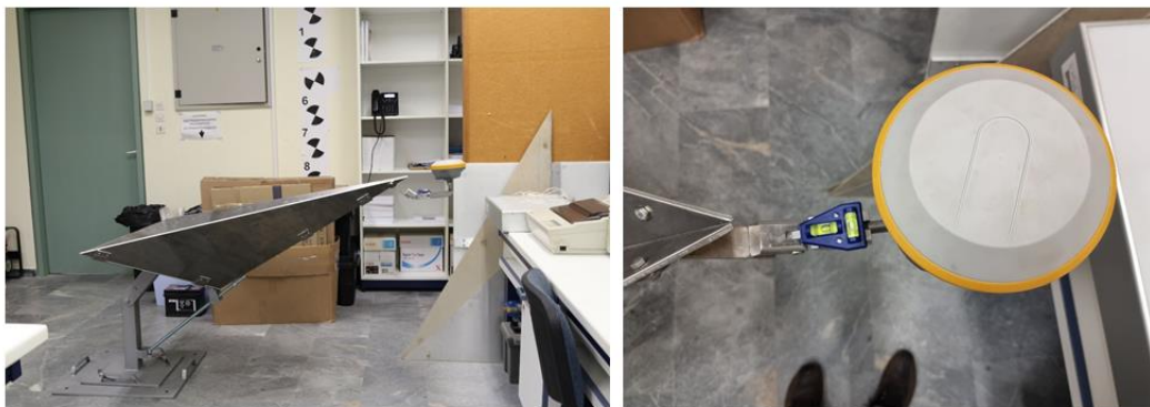
Figure 3. a) Mounted GNSS antenna in a horizontal position with the baseplate of the reflector at 80 degrees, b) Leveling of the GNSS antenna in three axes.
