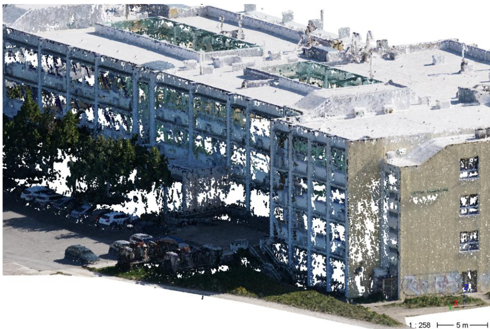
Figure 6. UAV point cloud of the Department of Geology at the University of Patras (oblique view).
