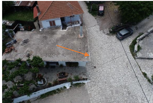
Figure 3: Low cost GNSS sensor installed on the roof of a building in the center of Krini village. The arrow shows the antenna.
