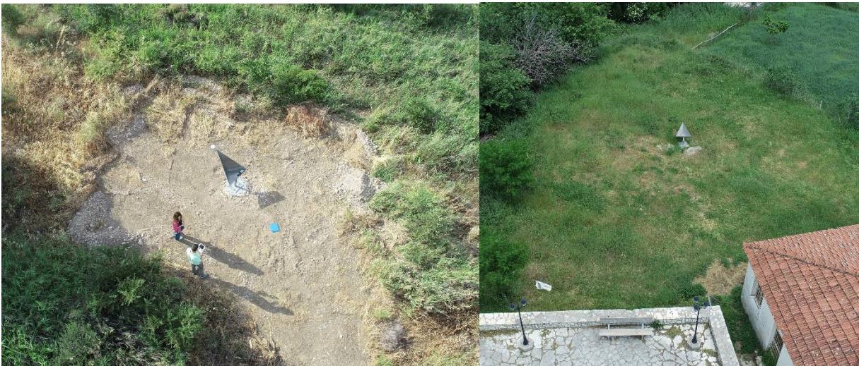
Figure 4. Persistent Scatterer (corner reflector) installation next to the Geology Department building. (b) Persistent Scatterer installation in Krini village.
